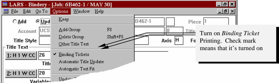
Figure 28 - Options Menu With Binding Tickets Print Turned On
